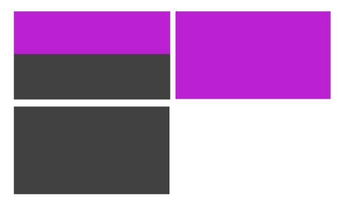
These Pathological patterns are very important pattern for SDI signal, because these 2 colors reveal the worst SDI signal, if the repeater or converter don't perform well, the jitter will be very high (bad). Sometimes the pathological pattern causes the monitor fail to receive signal. Please see the rp178.pdf file for the detail.
